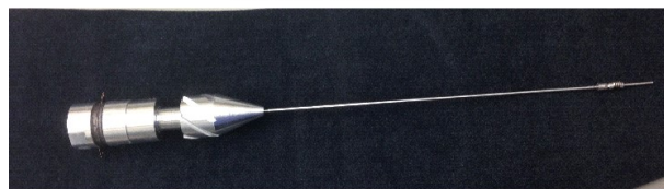
Fig. 2 Picture of the ultrasonic motor using transmission line and horn with oblique slits.
